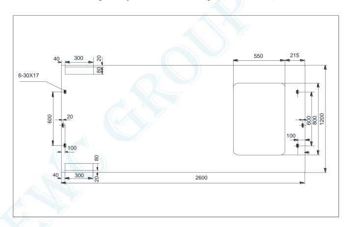
Figure 7/1 Open Pore Dimension of Switchgear Bottom Board
